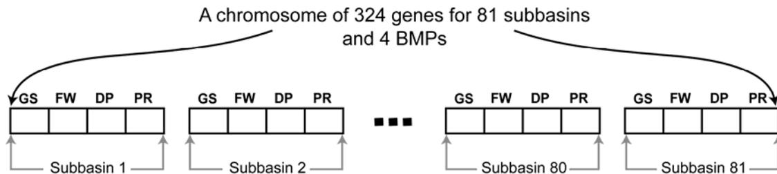
Fig. 6: Schematic of a chromosome in the genetic algorithm
