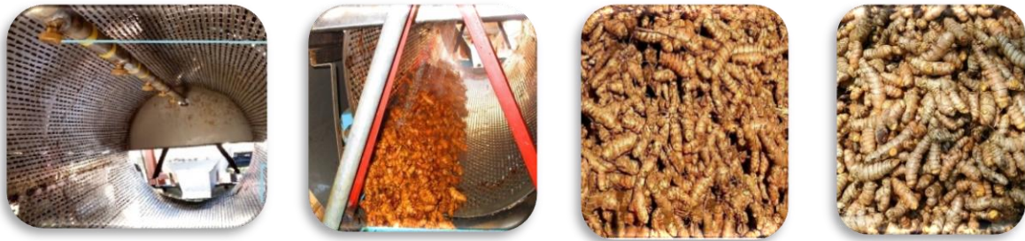
Fig. 5. Washing action and the initial and final conditions of washed turmeric
