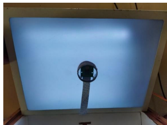
Fig. 2. Pi Camera module attached to the diffuser
