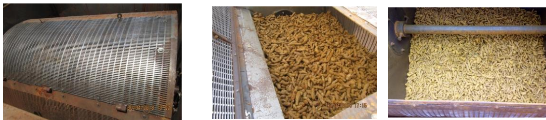
Fig. 7. Drying drum with raw and dried turmeric
