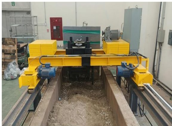
Fig. 1. Soil bin experimental setup showing the rail-mounted carriage in position.
