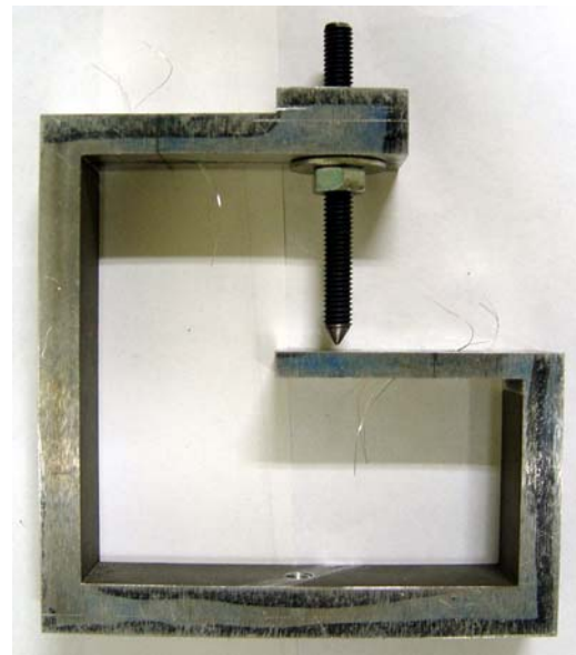
Fig. 2: A photographical view of the G-shaped load cell prototype
