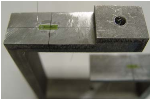
Fig. 6: The location of strain gage in the upper portion of frame A
